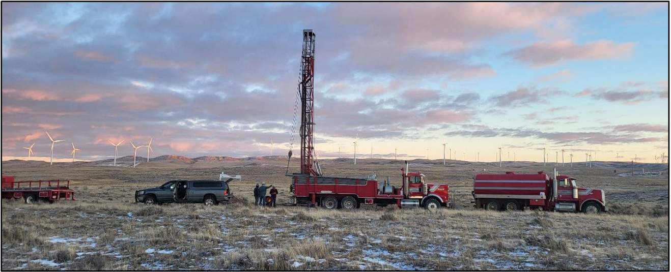
FIGURE 3: MUD ROTARY DRILL RIG AND GEOPHYSICAL PROBE TRUCK NORTH OF MINE UNIT 2
