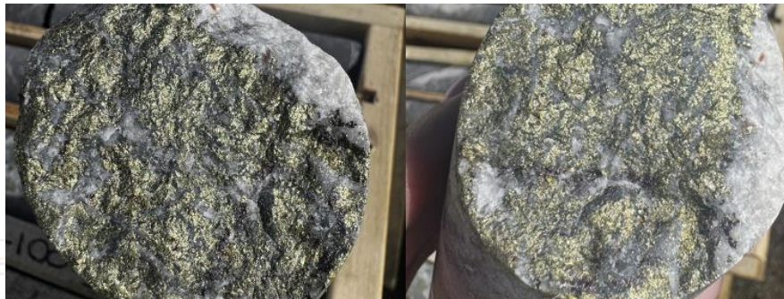
Chalcopyrite-bornite-quartz-carbonate veining below the base of the sedimentary structure in STK25001 at 291.4m that returned assays of 14.95% Cu & 0.51g/t Au. Core diameter is NQ2
