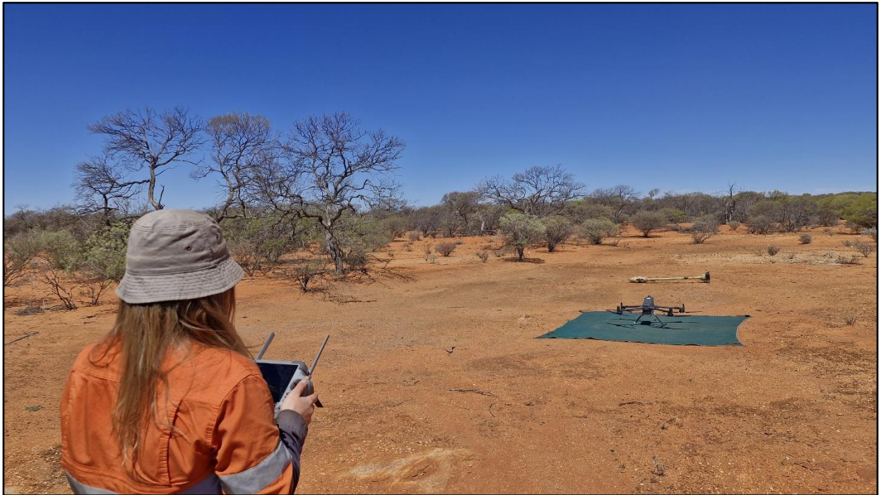
Figure 1: Survey team from Pegasus Airbourne undertaking high-resolution magnetic survey at the Austin Gold Project.
