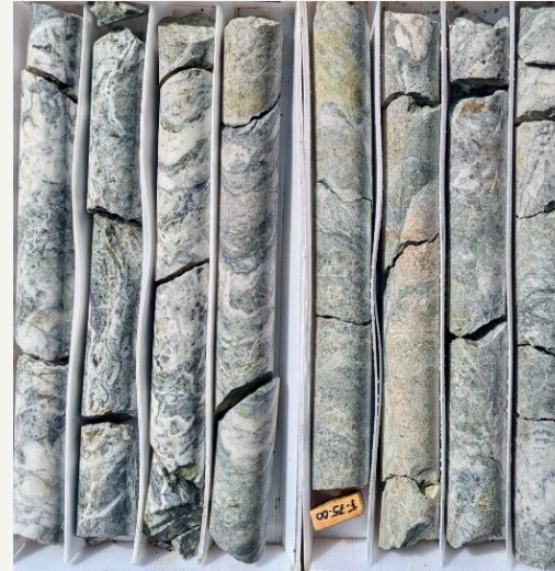
1 Banded quartz vein in drill core. CDH-152: 1.98m @ 4.59 g/t gold, 520 g/t silver from 18.5m (left) and CDH-154: 1.90m @ 1.83 g/t gold, 305 g/t silver from 75.1m (right).
