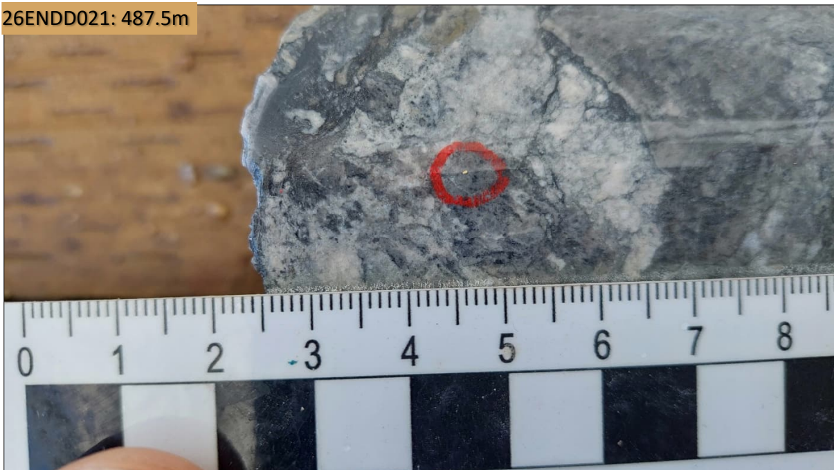
Photo 5. Visible gold (circled red) in hole 26ENDD021 at 487.5m down hole in brecciated quartz-carbonate-pyrite-arsenopyrite veins within brecciated/faulted granite. Numerical units on scalebar are centimetres.
