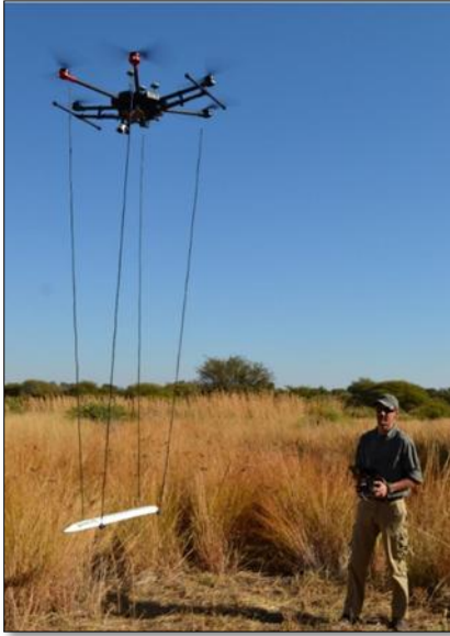
Figure 3. MagArrow sensor and drone used for magnetic surveys on the Garies tenement.
