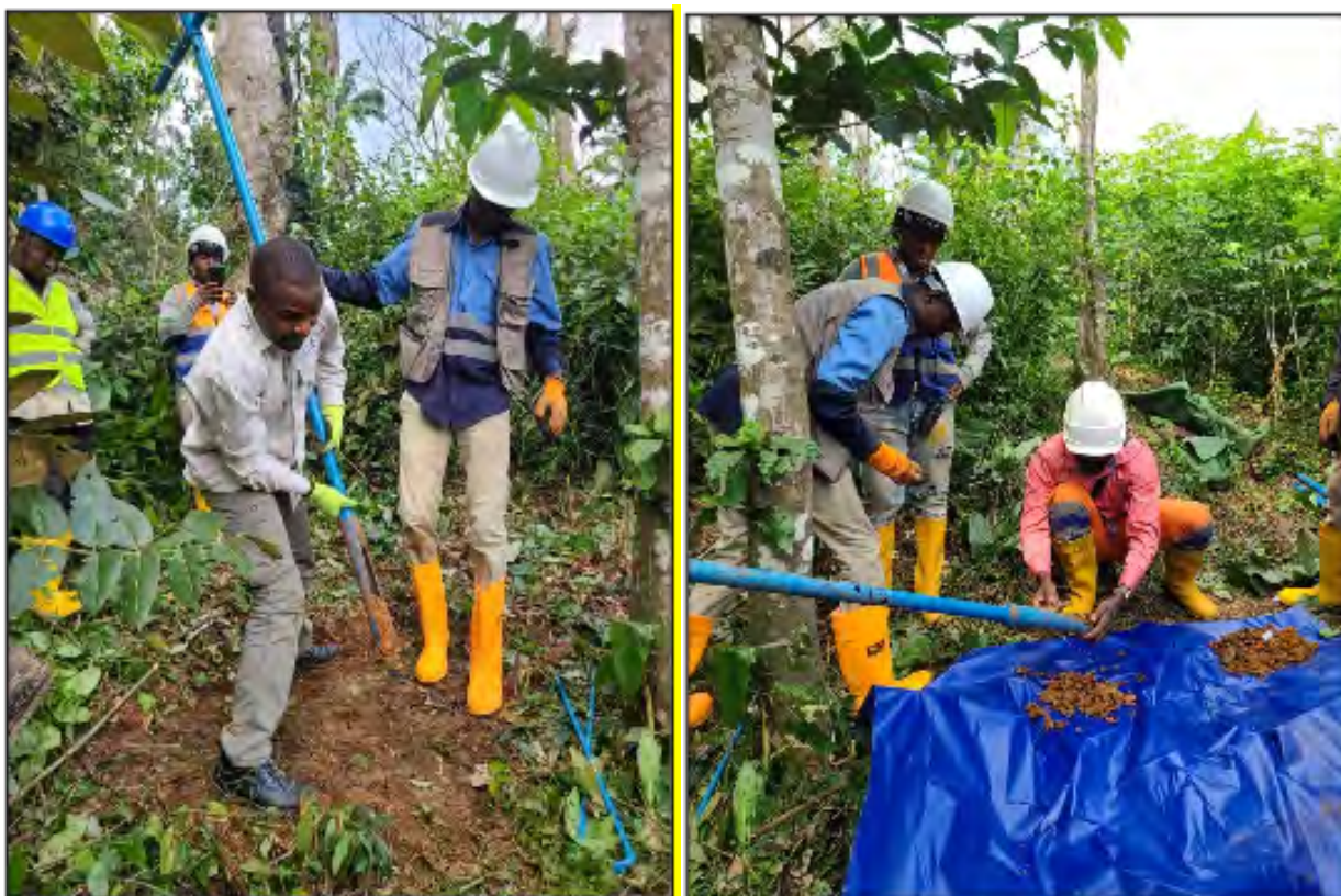
Figure 4. Tusker Minerals hand auger drilling activities showing sample collection process.
