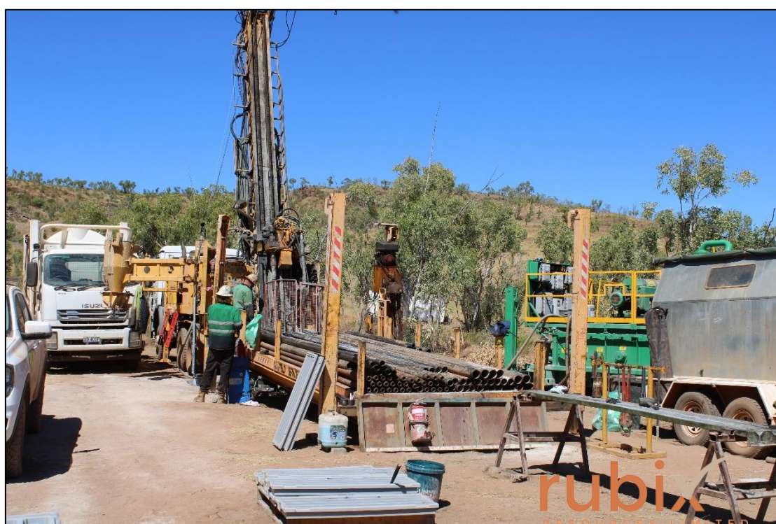
Figure 2 – Drilling at Grunter North using a multipurpose RC/DDH rig (UDR650). Green unit to the right of the rod truck is the centrifuge, which separates fines from water for recycling during drilling, significantly reducing the water requirement of drilling unless circulation is lost downhole.
