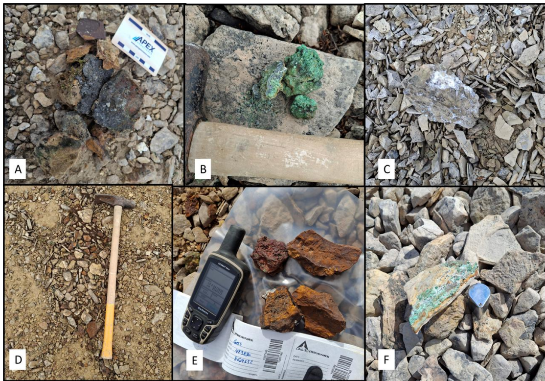
Figure 10: Examples of the interpreted copper gossans and outcrop from the Storm-Tornado area. Portable XRF was used to aid visual identification and these samples have not yet been analysed by laboratory.
