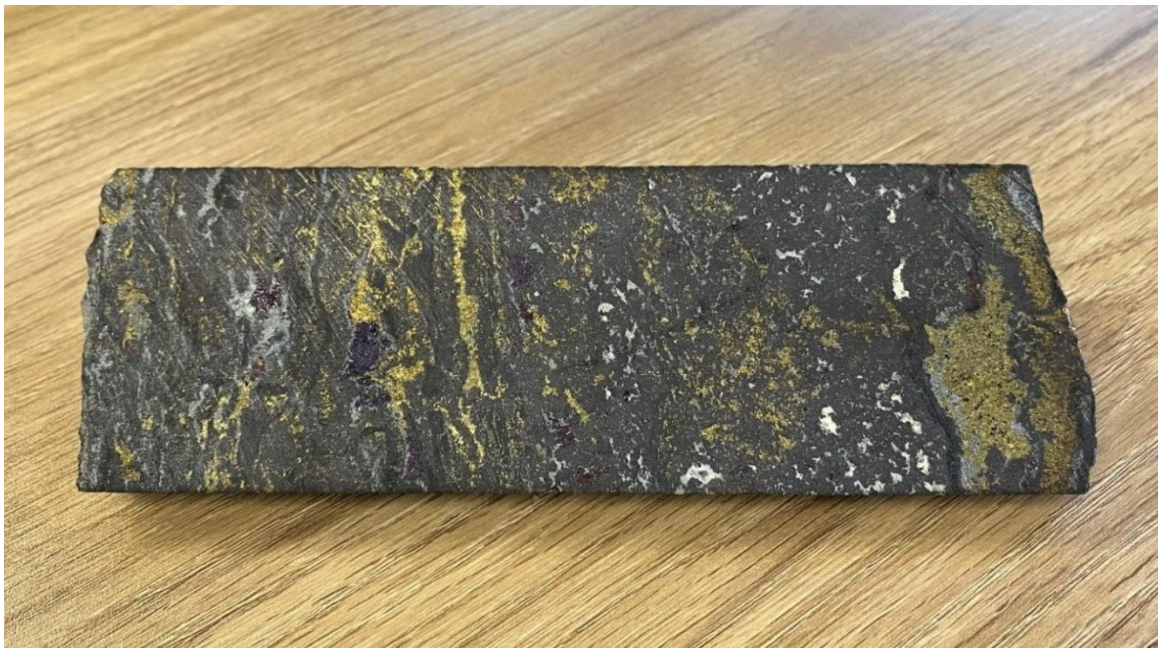
Figure 15: Drill core from previously released diamond drill hole WD22-01 from approximately 544m (1,785ft) downhole from the ‘Goldilocks Zone’ which assayed 95g/t In, 2.8% Cu, 0.5g/t Au, 39g/t Ag.
