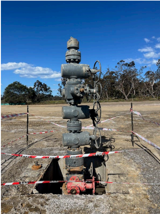
Figures 3 & 4: Wombat-5 production wellhead and cleared wellsite
