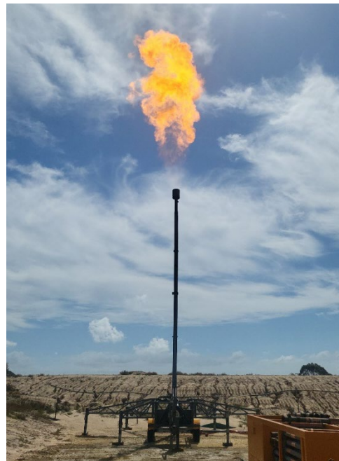
Figure 2: Wombat-5 gas flare on 19 January 2026, following blowing down with Nitrogen
