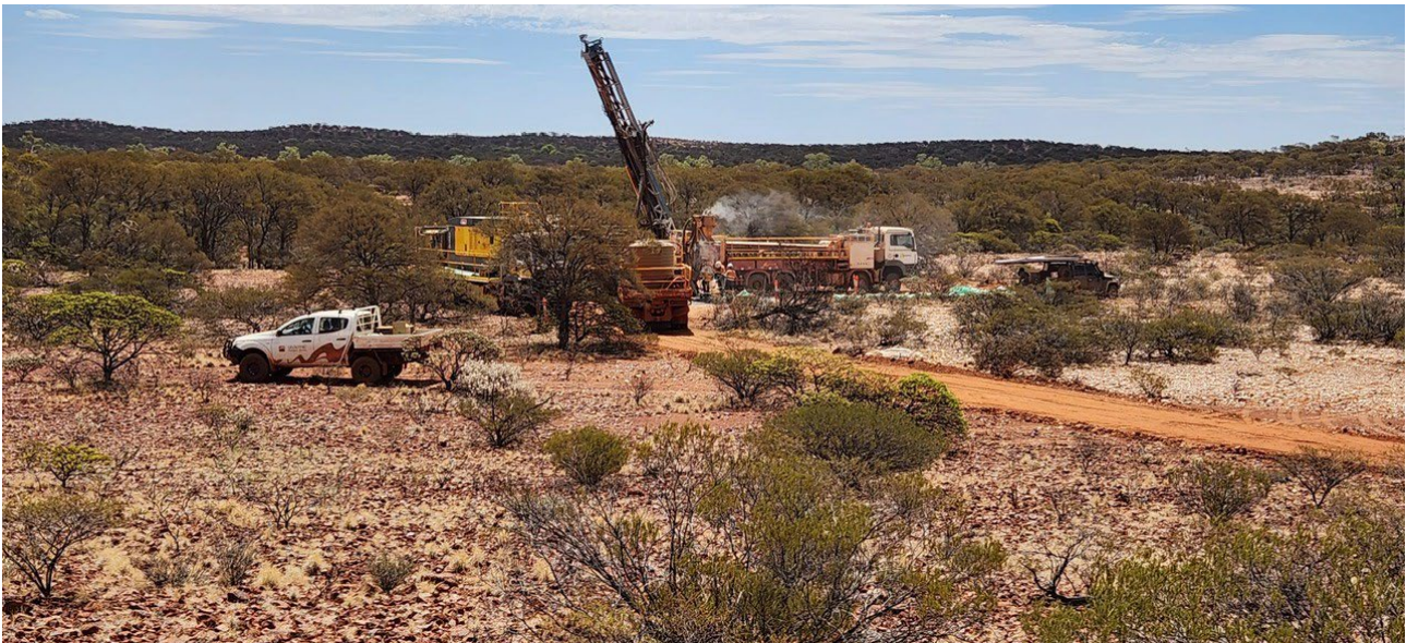
Figure 2. RC rig set up on the first Degrussa West drillhole testing soil anomalism. Quartz veining in Peak Hill Schist outcrop seen in foreground.
