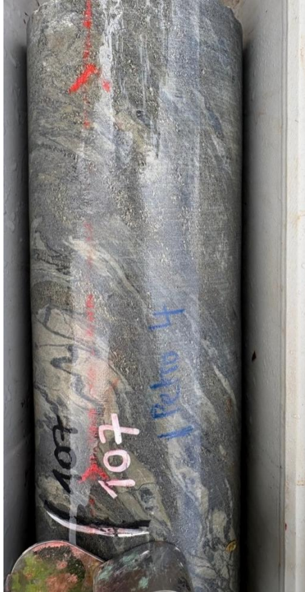
Figure 2 – Mt Stirling Hole 26MSDD001 - View of Core at 107.00-107.18m depth where 1m interval from 107m returned 22.6 g/t Au
