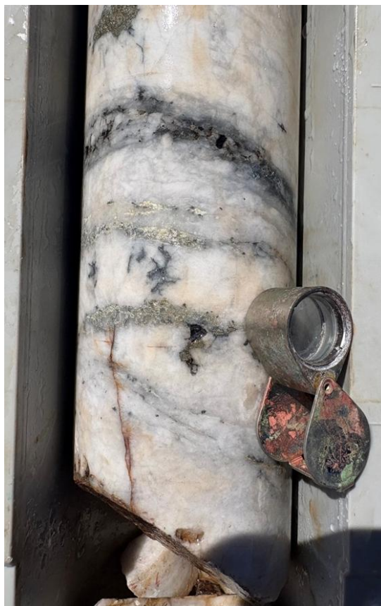
Figure 4 – Mt Stirling Well Hole 26MSDD003 - View of Core at 48.27-48.5m depth where 0.77m interval from 47.9m returned 30.2 g/t Au
