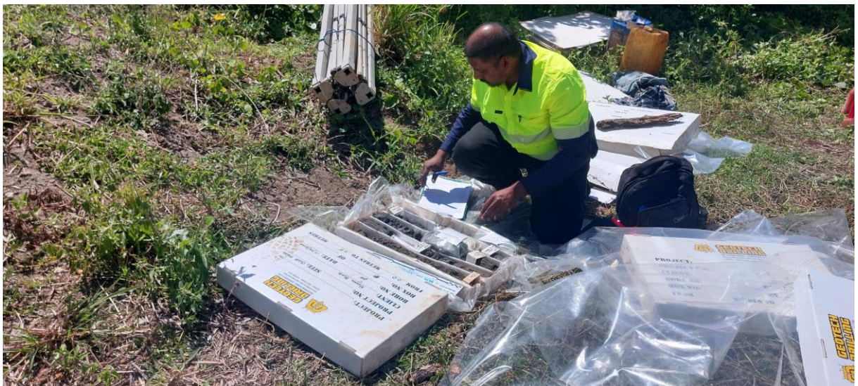
Plate 8 – Sand core samples being logged and packaged for shipment to the laboratory
