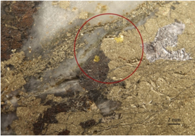
Drill hole CT9004 Visible gold flakes hosted in sphalerite (dark grey) and on the boundary between quartz and pyrite. These two grains are contained within the interpreted western extension of the C03 structure referred to in the 2012 resource and reserve report. The structure is identified as C03W.
