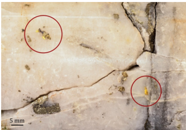
Drill hole CT9004 Visible gold grains within the C38 structure.
