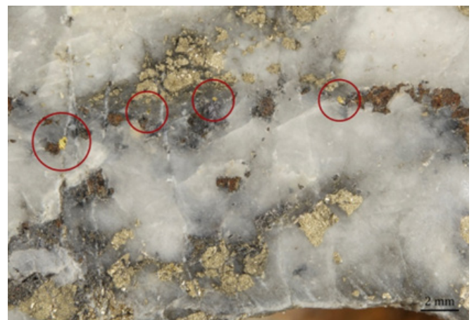
Drill hole CT9004 Visible gold grains within drill core from the C38 structure.
