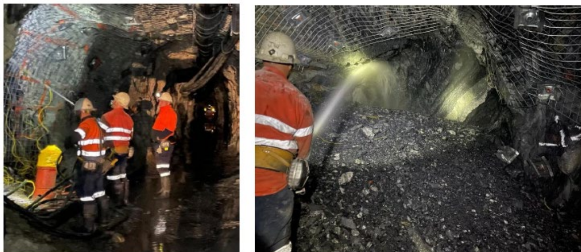
Image 5: "Star of Peace" Reef being charged up and house down the ore, post blasting
