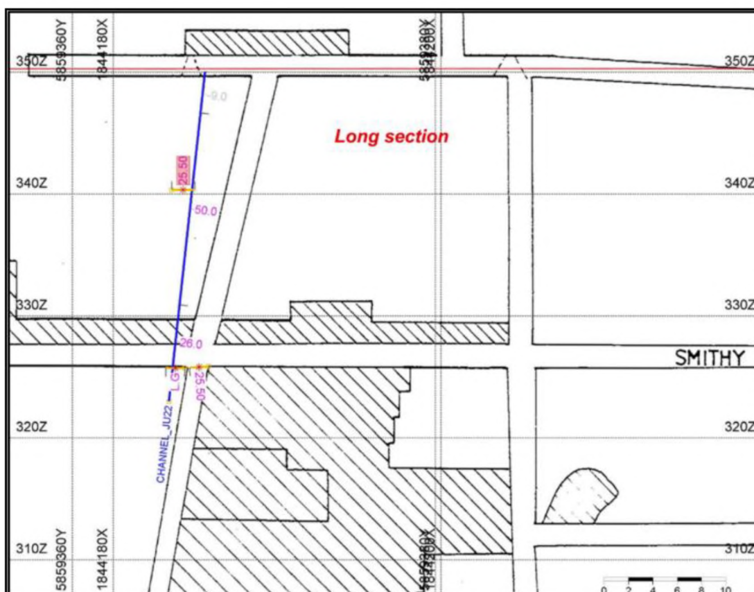
Figure 5: Channel_JU22: 23.0m @ 42g/t Au is a rise channel or vertical in the Long Section of the Jubilee mine
