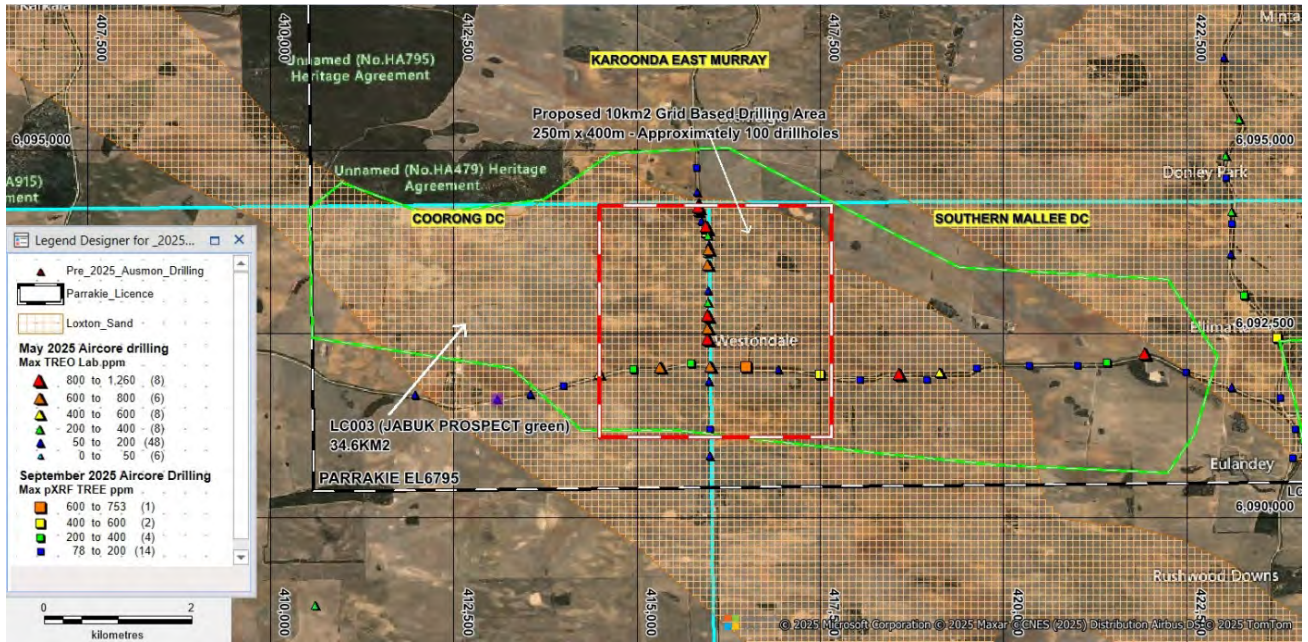
Figure 5: Jabuk Prospect showing the most recent (September 2025) road verge drilling, significant TREE intervals and proposed close spaced grid drilling area (broken red line boundary).
