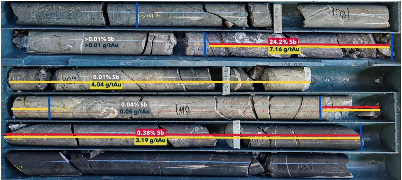
Figure 3: Photo of the core from drillhole DD25ZOP014 showing distribution of the mineralised zone with high-grade antimony and gold grades.
