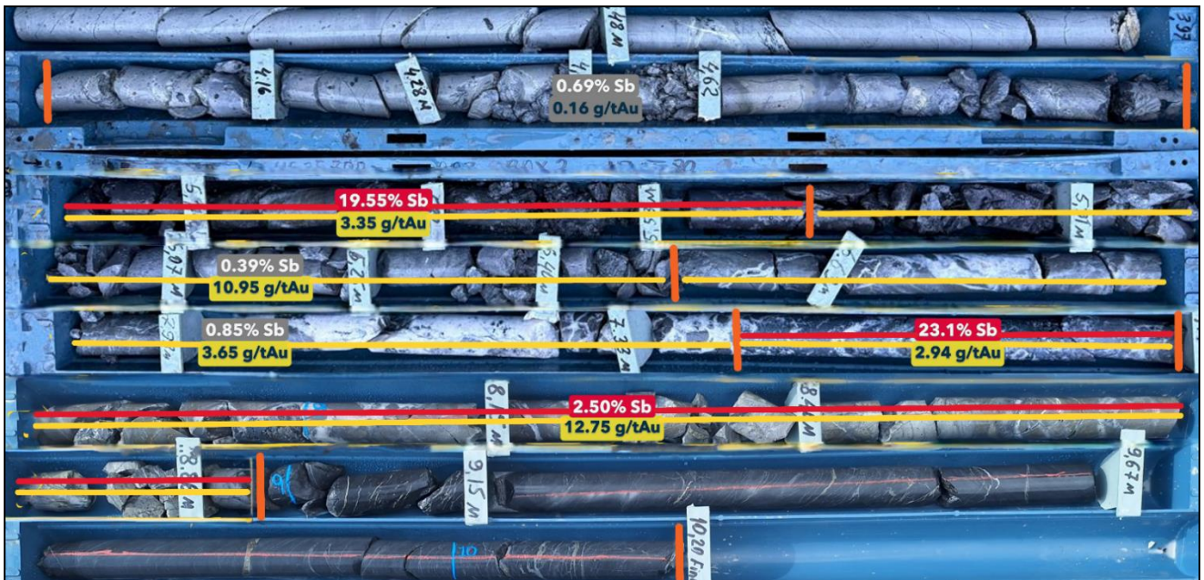
Figure 4: Photo of core from drillhole UG25ZOP003 showing distribution of sample intervals and high-grade assay results
