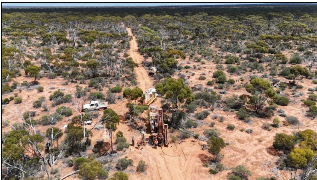
Figure 4: Aircore drilling during the campaign at the Torquata Prospect
