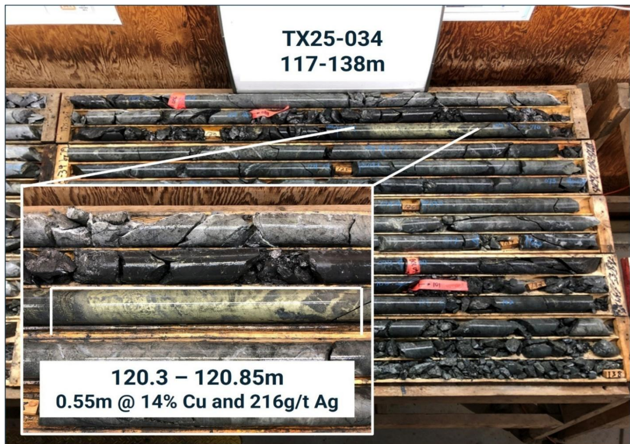
Figure 4: Diamond Drill Core showing high-grade massive chalcopryite intersection from drill-hole TX25-034
