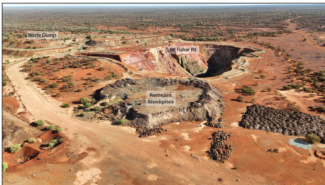
Figure 4: Mt Fisher Mine looking north-west showing historical pit, waste dumps and tailings storage facility.
