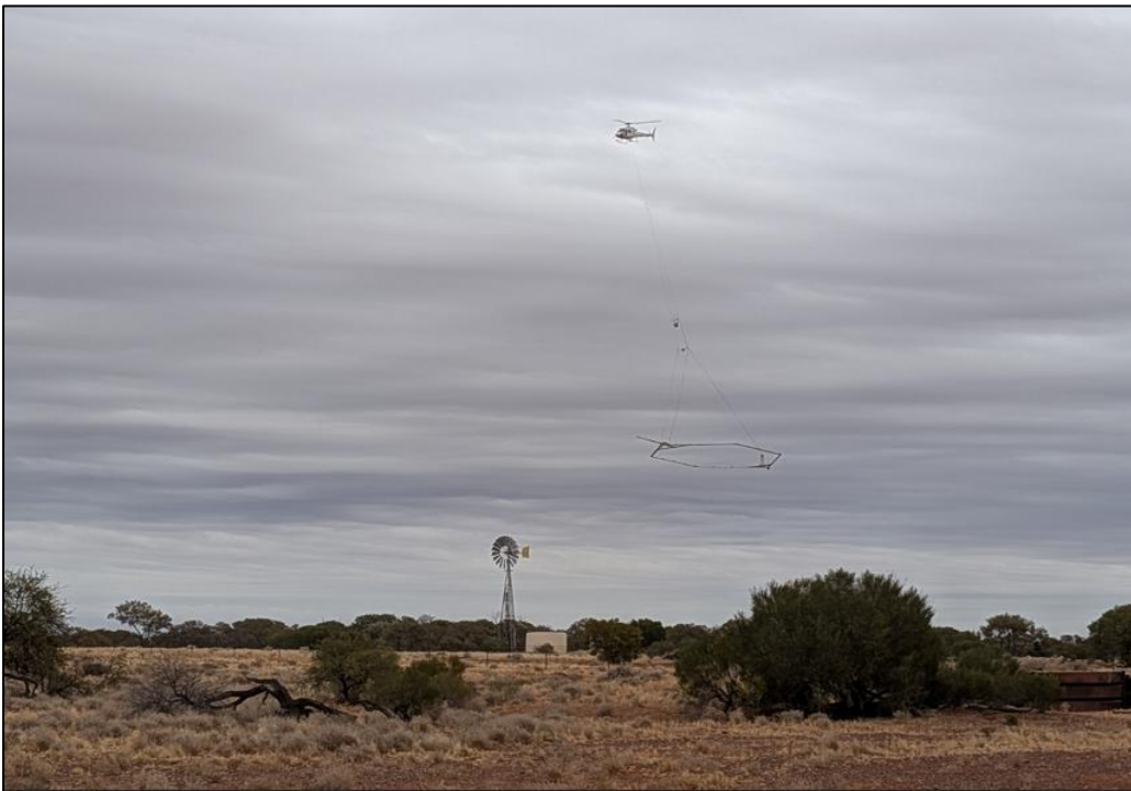
Figure 7: Helicopter acquisition of high-resolution SkyTEM Airborne EM survey data over the Marymia East project.
