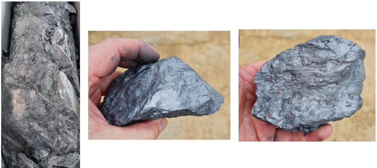
Figure 16: Graphite from the Burke Deposit recovered from core drilling (2023)
