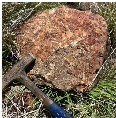
Stockwork quartz-potassium feldspar veining (at 217903mE, 7372231mN)
