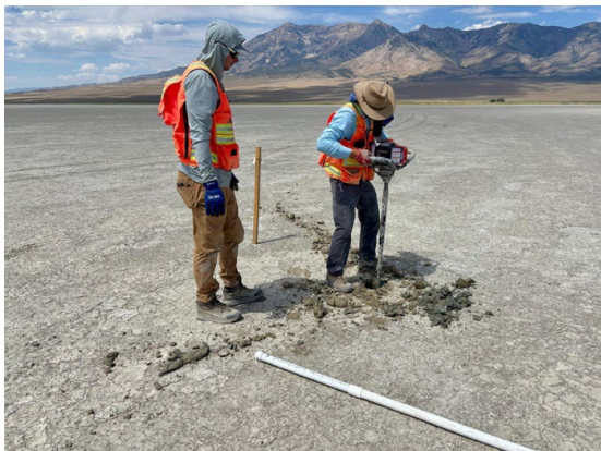
Figure 23: Auger Sampling at White Plains
