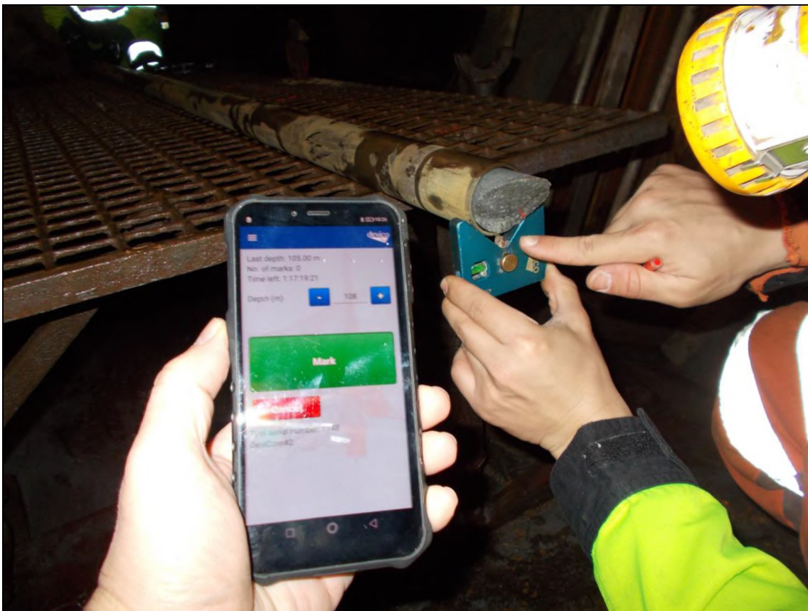
FIGURE 10-4: PROCESS OF CORE ORIENTATION AT UNDERGROUND DRILL SITE BY A DRILLER USING DEVICORE INSTRUMENT
