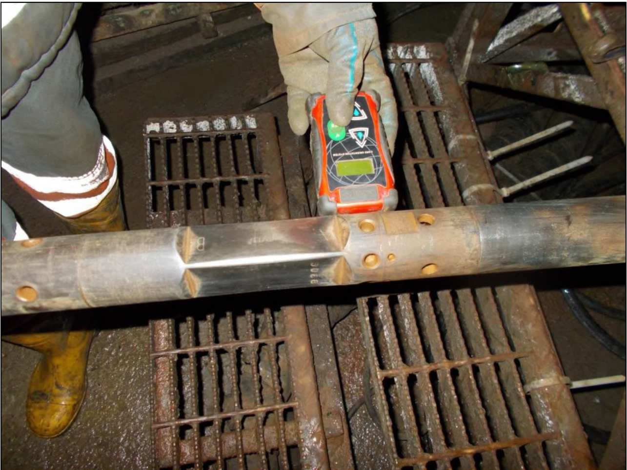
FIGURE 10-3: PROCESS OF CORE ORIENTATION AT UNDERGROUND DRILL SITE BY A DRILLER USING ORIFINDER CONTROLLER
