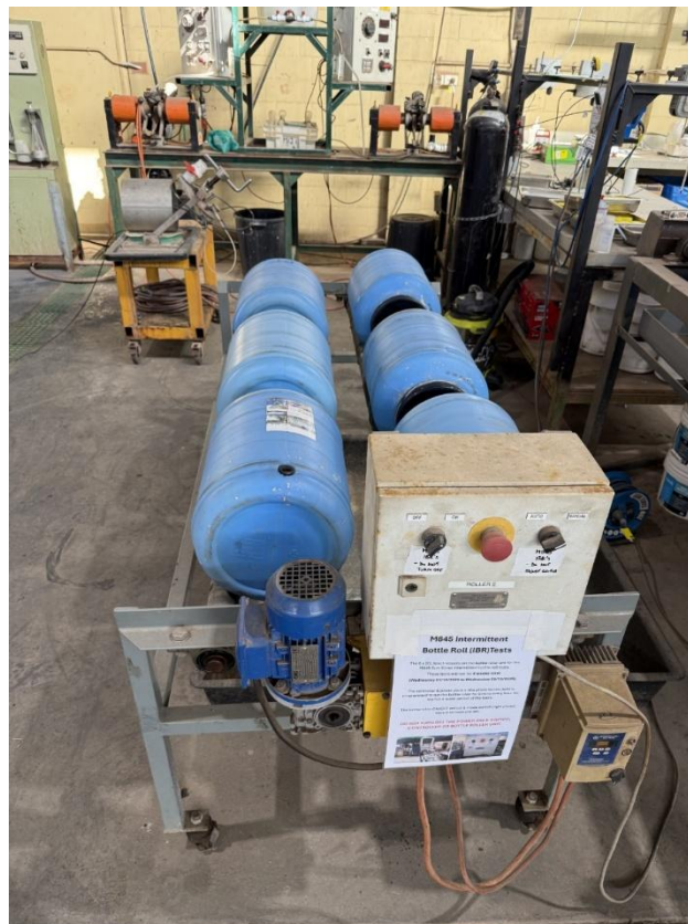
Figure 8 – IBR Metallurgical Testing two sample composites three grind sizes (6.3mm, 3.35mm, 2mm)
