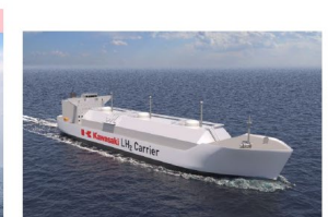
Concept image of 40,000m3 scale liquefied hydrogen carrier (Image provided by Kawasaki Heavy Industries, Ltd.)
