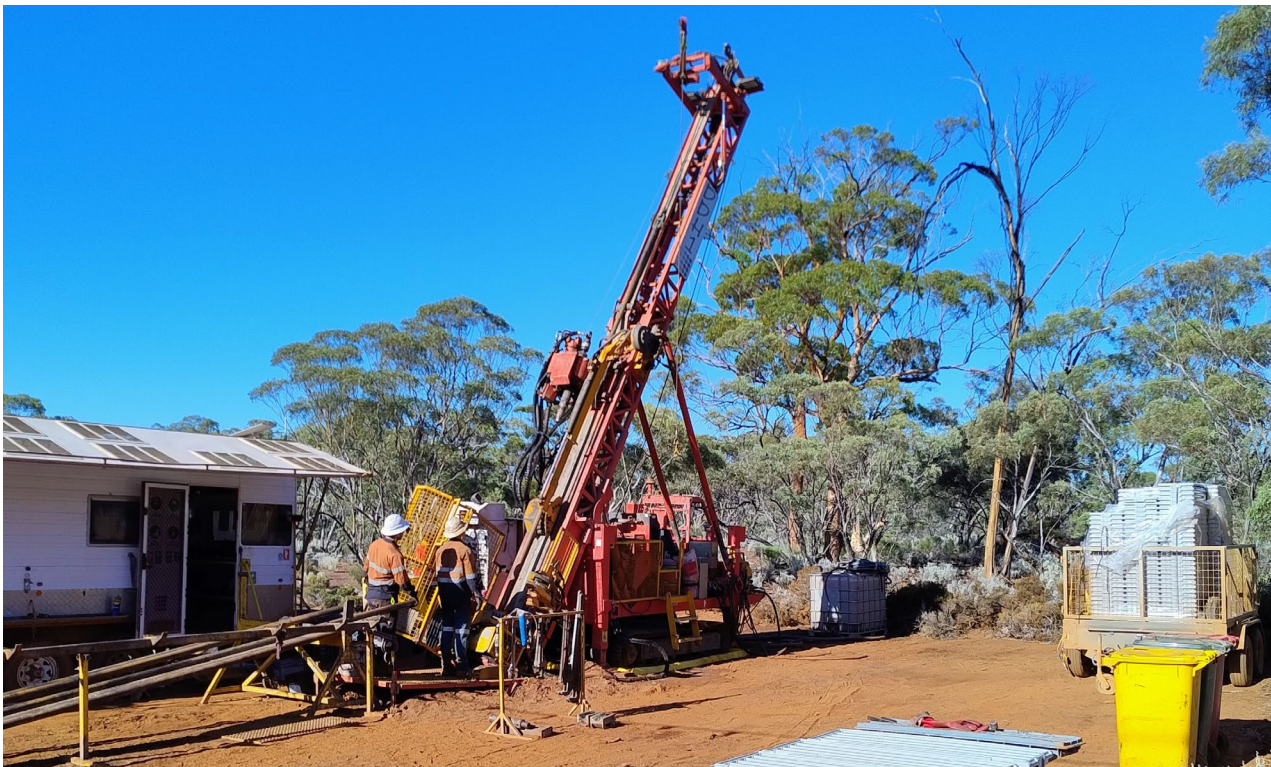
Figure 1: Diamond drill rig at Cognac West, March 2026
