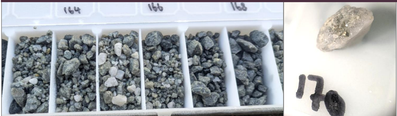
Figure 8. RC chips from SJRC003, highlighting a zone of strong sulphide alteration and quartz veining. and quartz veining.
