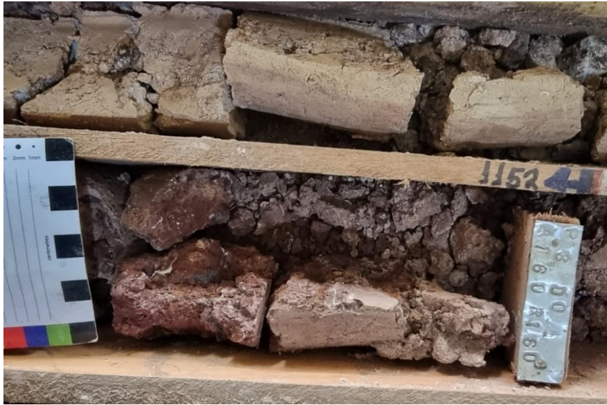
Figure 2: Half drill core from MFSR-44 with downhole direction to the right. Material in the lower row is the end of sample 1152 to 8m downhole (wooden block with tag, bottom row of photo). The top row is the clay-rich fraction, approximately 7m downhole. The lower row reddish material is strongly magnetic with 12.9 \times 10^{-3} SI Units. This material is all part of sample 1152, which reported 2m at 8.56% TREO from 6m (see Table 1). Scale is in cm.
