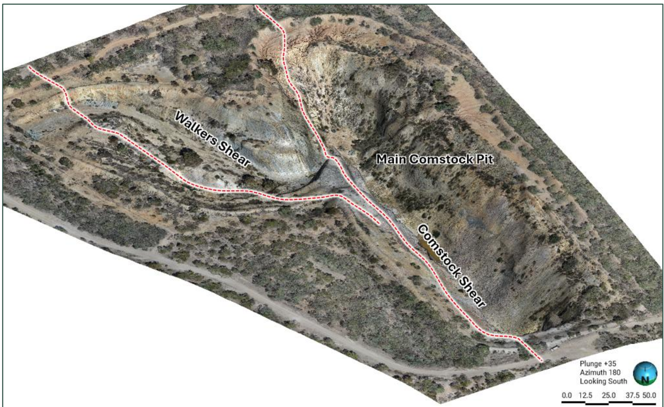
Figure 1 – View of the high-accuracy LiDAR and photogrammetry of the Comstock open-cut pit – looking towards the South (azimuth 180). The main Comstock Shear Zone and Walkers Shear zone are highlighted. Current entrance to the pit is possible from the Walkers Shear side.
