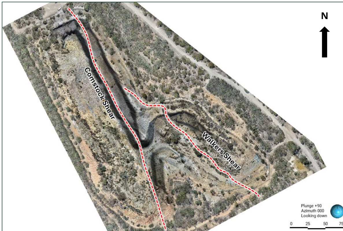
Figure 4 – View of the high-accuracy LiDAR and photogrammetry of the Comstock open-cut pit with key projected structures – looking down.
