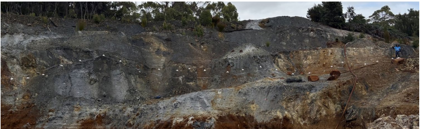
Photo 1. Systematic channel sampling at the Granville East pit
