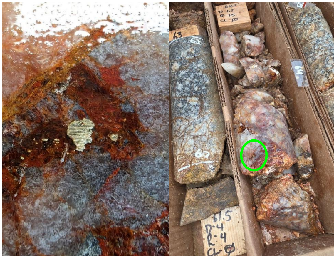
Figure 1: ~30 cm of a massive quartz-sulphide (30%) vein returned 0.61m @ 71.9 g/t Au, 92.5 g/t Ag from 19.2m. Oxidation of sulphides to goethite–limonite–hematite with native gold preserved as ragged/leafy grains spatially associated with the iron-oxides.
