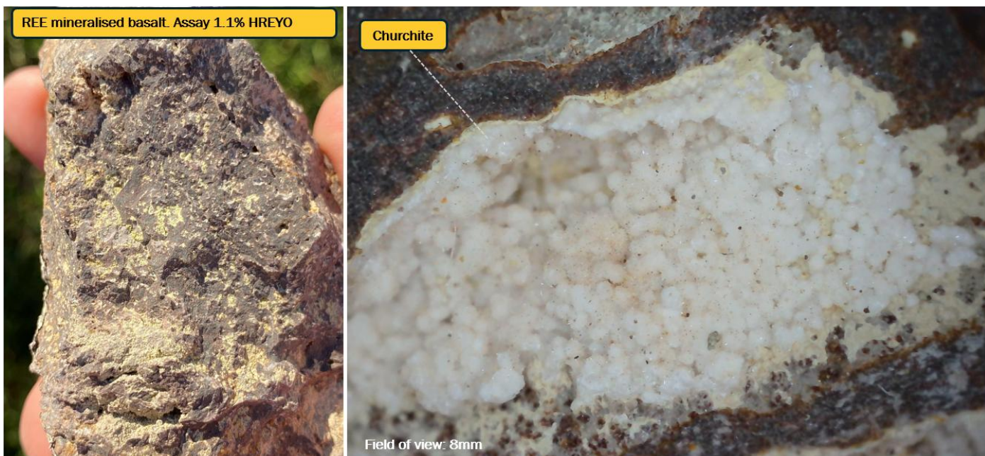
Figure 2 Left: basalt clast from within a polymict breccia containing secondary (supergene) heavy rare earth minerals churchite and xenotime: sample collected in 2023. Right: reflected light microscope photo of churchite in a void within a vesicular basalt breccia clast from the same sample.
