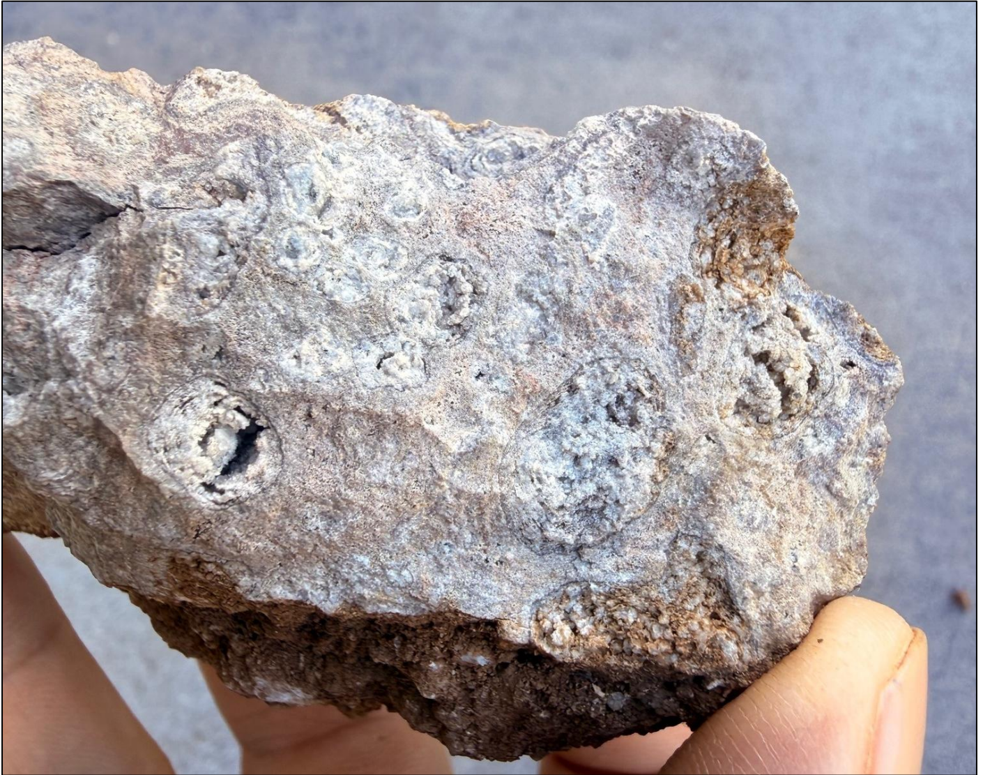
Figure 1 Spherulitic rhyolite (sample GG1RK1011) which assayed 2230 ppm HREYO and is interpreted to be magmatic REE mineralisation.
