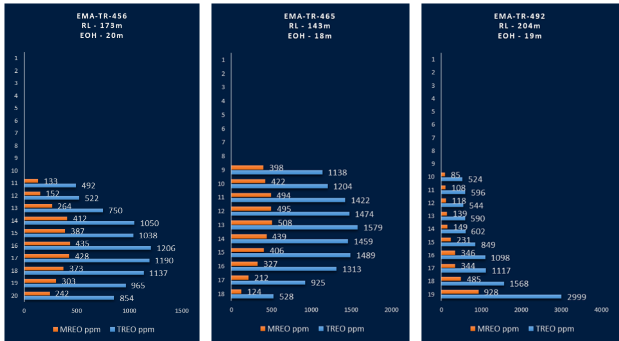
Figure 4 – Drill-hole profiles showing typical ionic REE enrichment zone with high NdPr grades close to the fresh rock interface.
