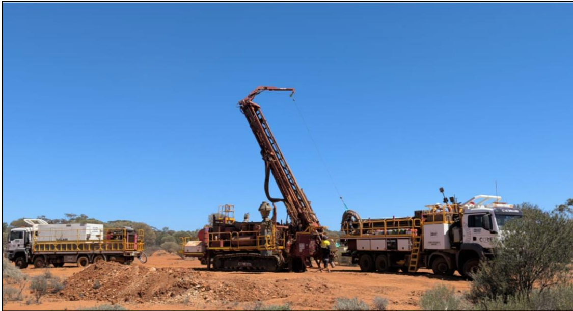
Figure 1. RC drilling underway at Breakaway Dam (Core Drilling Pty Ltd rig)
