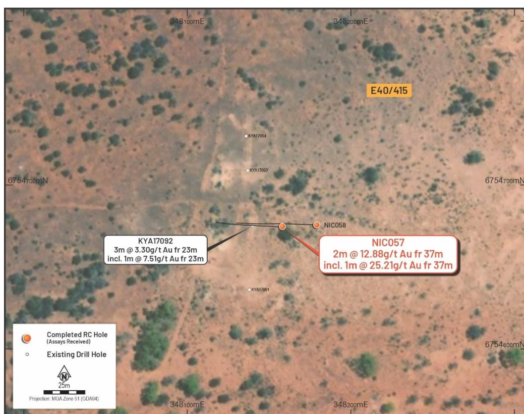
Figure 1 - Plan View of Drilling at Woodpecker
