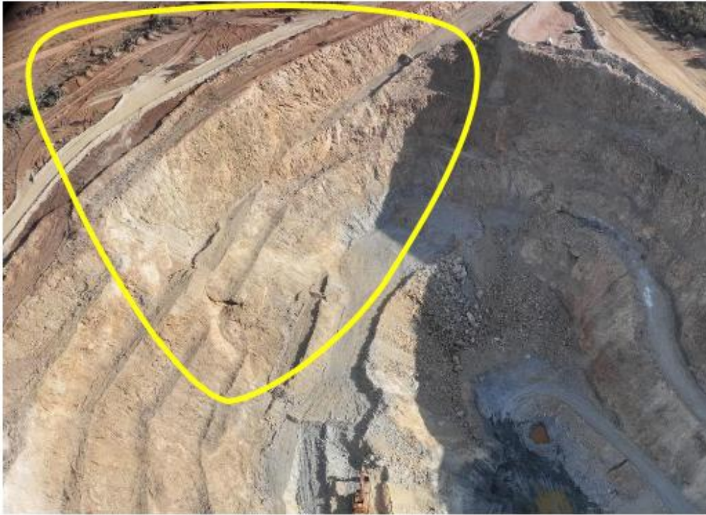
Figure: Pearse South (looking north) as at 12 January 2026. The rehabilitated section of the wall is highlighted in yellow. Ongoing monitoring is underway on the North and Western walls.
