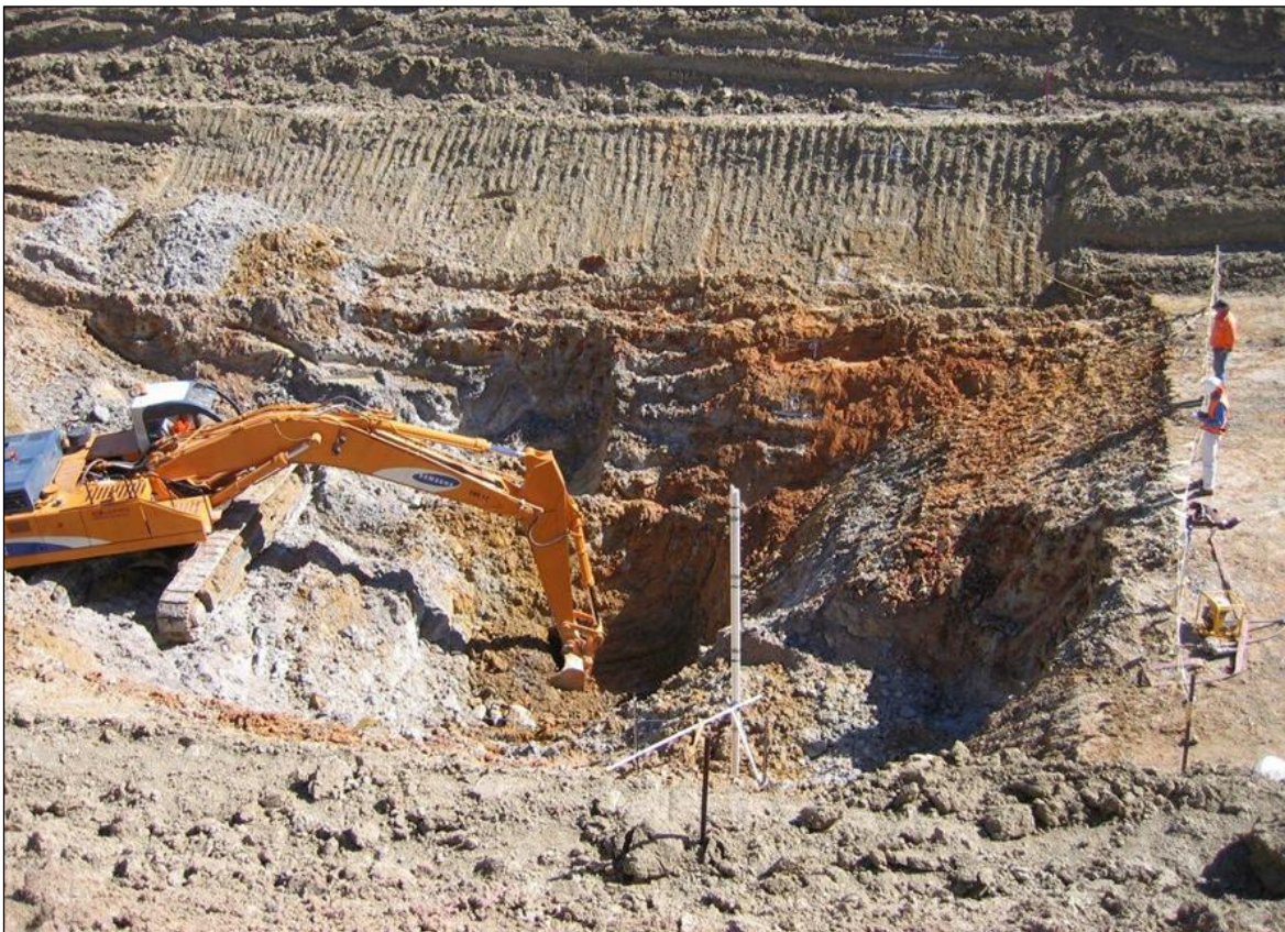
Figure 16.5 Test pit ore excavation trial showing extraction of ore zone
