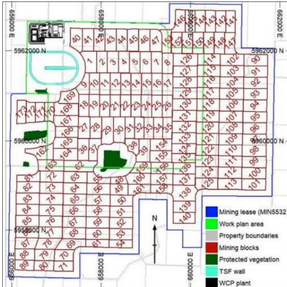
Figure 16.6 LOM schematic showing final mine plan with mining block sequence and the position of fixed infrastructure within MIN5532 and the Work Plan area
