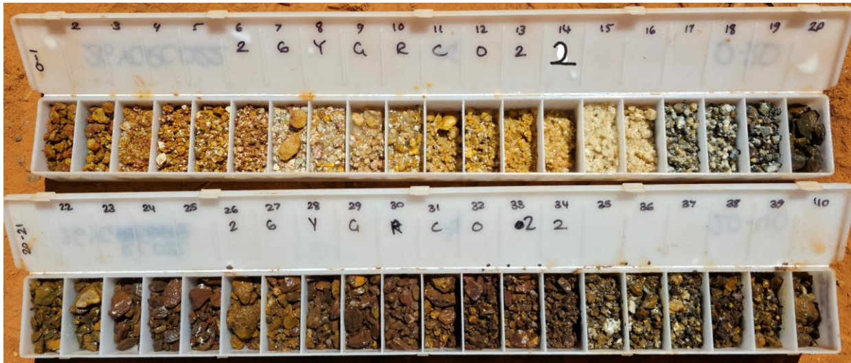
Figure 4. Representative RC rock chip samples from drill hole 26YCRC022 (0-40m (EOH)), Chicken Little.
