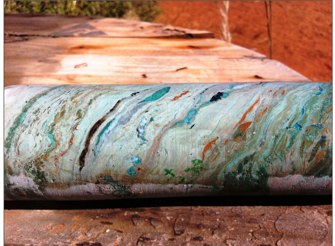
EPT604 – Copper mineralisation at Tyrell – part of 6.6m @ 2.8% Cu from 34.8m*
