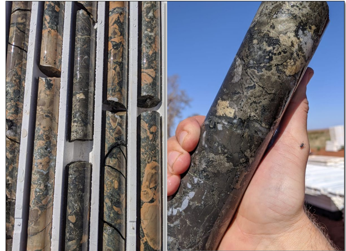
ETG0203 – Photo 1 (~185-190m) Brecciated and altered sediments containing disseminated and blebby sulphides. Photo 2 (~187m) Coarse euhedral pyrite and fine pyrite alteration within silicified and brecciated sediment
