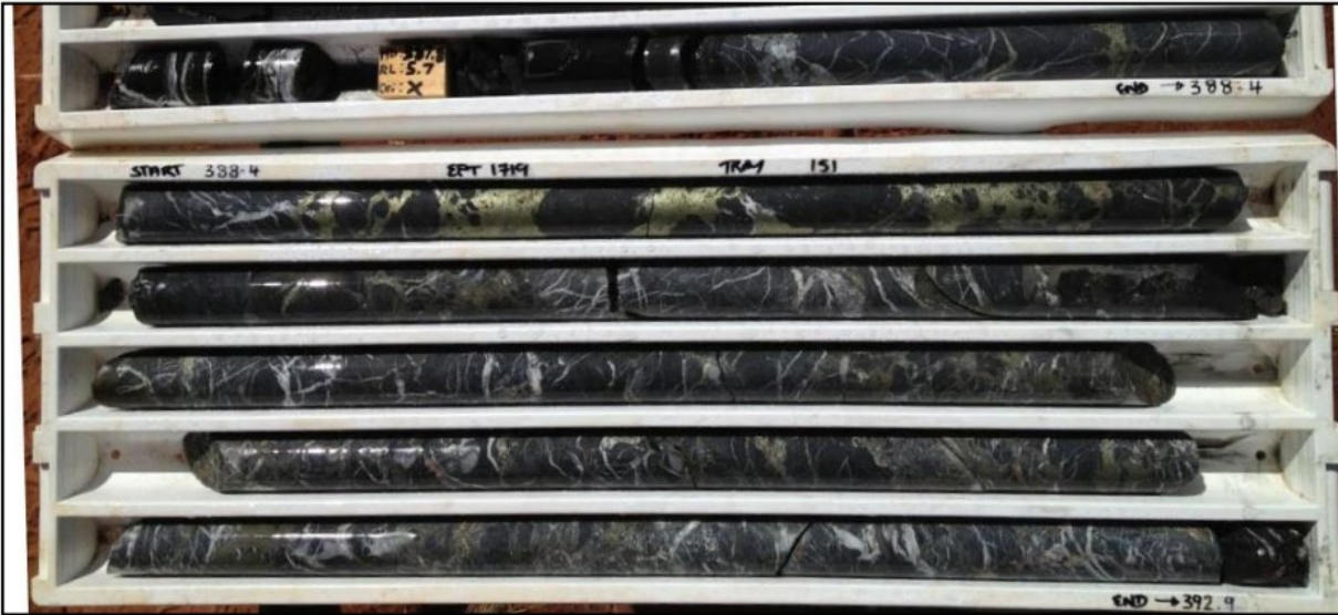
EPT1719 - ~387.6m to 392.9m (5.3m @ 2.5% Cu) – Veined and brecciated carbonate with local massive copper sulphide
