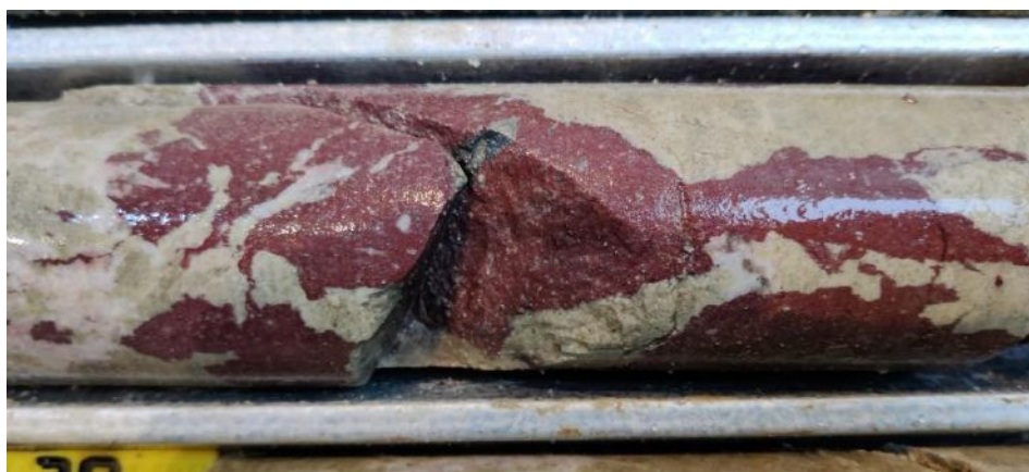
Figure 6: Bastnäsite-bearing carbonatite (GD003, 101.4 m). Core section showing disseminated to patchy bastnäsite mineralisation (~25 %, red) within a carbonate matrix (~75 %, beige) composed mainly of calcite and siderite. Minor hematite occurs along fractures and grain boundaries. Rare-earth mineralisation is visually estimated.
