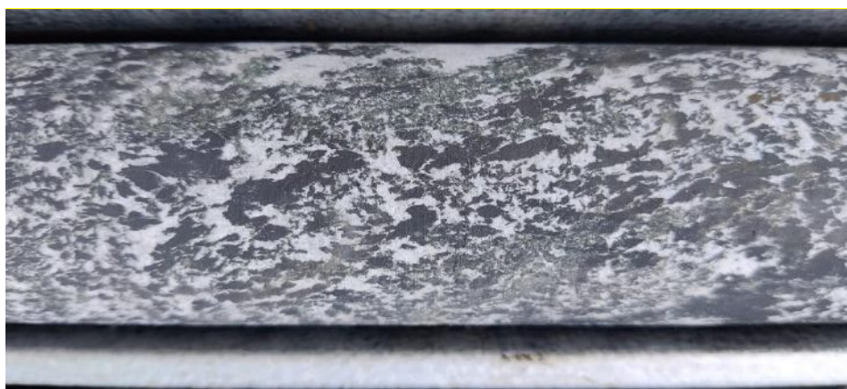
Figure 7: Magnetite-Altered Carbonatite (GD001, 182.4m) Core interval showing disseminated to banded magnetite (~40 %, black) hosted within a carbonate matrix (~60 %, white) composed predominantly of calcite. Magnetite occurs as subhedral grains and veinlets overprinting the carbonatite. Visual estimates are qualitative only.
