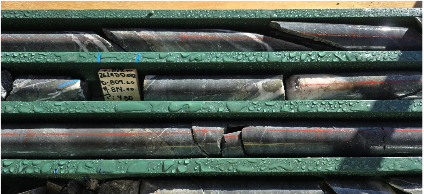
Photo 2. Zone of intense pyrite-chalcopyrite-quartz vein style and fine disseminated mineralisation from 809m downhole in 26LHDD072* (refer to Appendix 1).
