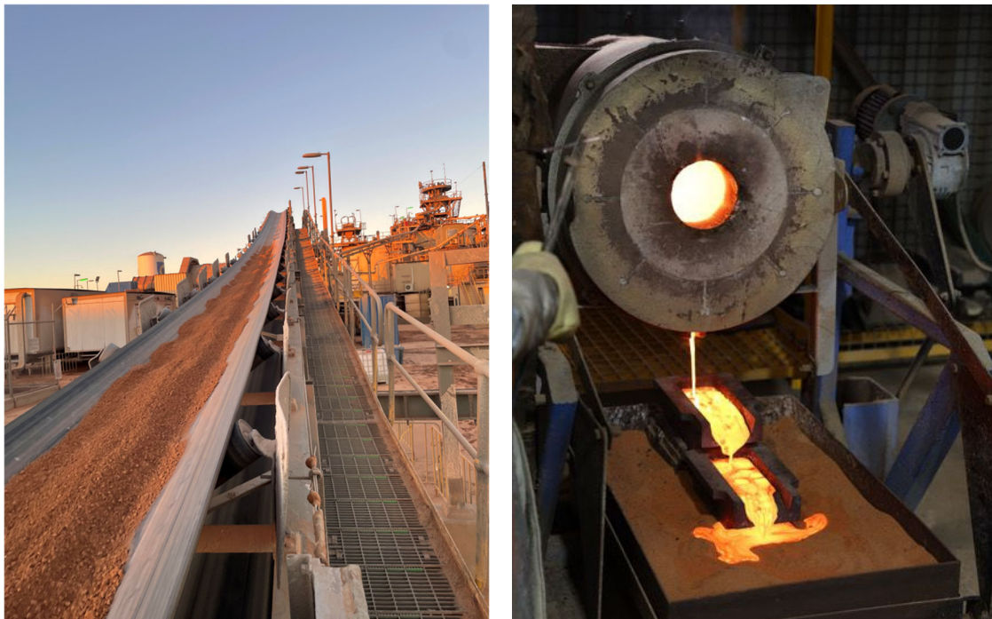
Figure 1: First Fingals Ore on the main conveyor at Lakewood and first gold pour from the Fingals and Majestic mines.
