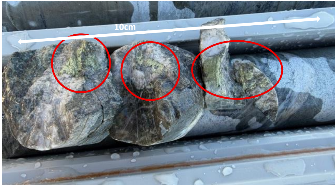
Photo 1: Select core with visible chalcopyrite blebs in quartz veining at 183.6m MBDD001
