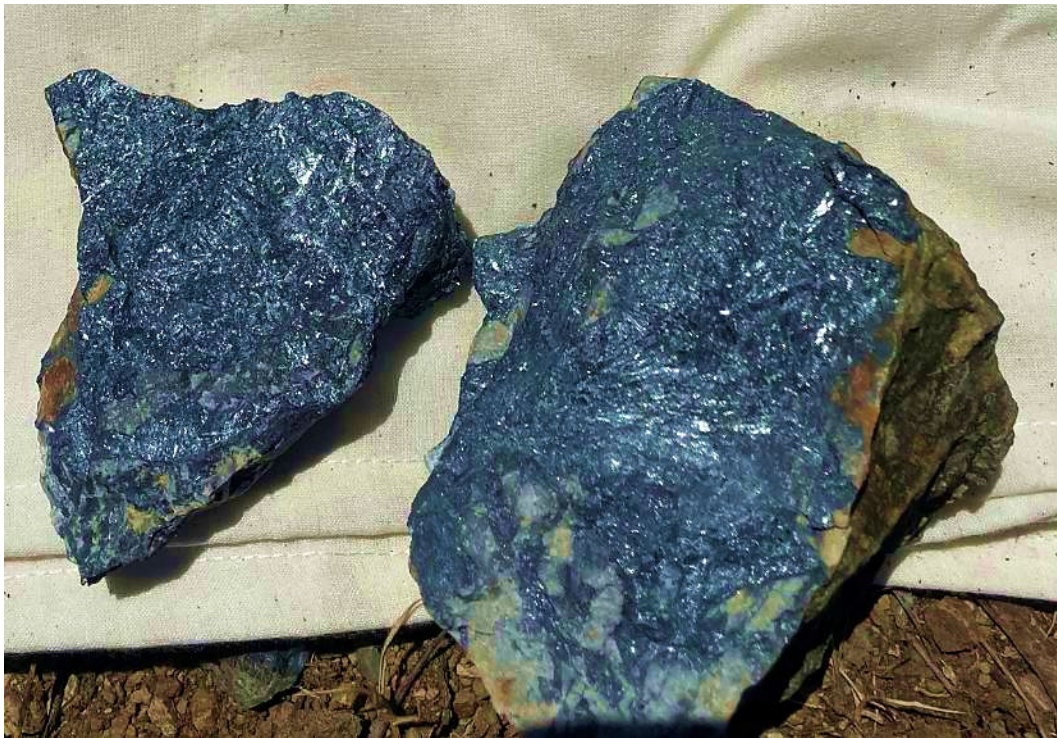
Photo 2. Sample R571 – Stibnite-Quartz breccia grading 31.5% antimony (Sb)
