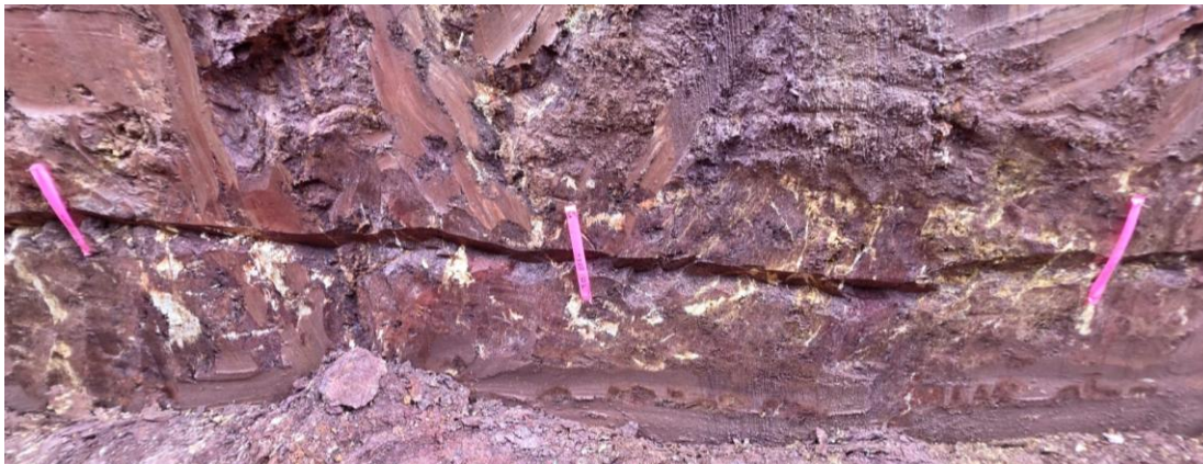
Figure 3: Trench 2 ending in the western border in highly fractured and sheared mafic volcanics at 215.5m.
