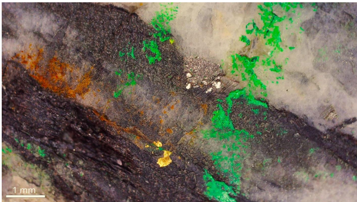
Figure 4: St Arnaud Comstock visible gold (25NED007) and pyrite. Note, the green colour is residual chinagraph pencil markings from the logging process.
