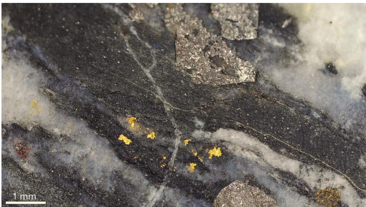
Figure 5: Microscope image of core containing visible gold and pyrite 25NED007.
