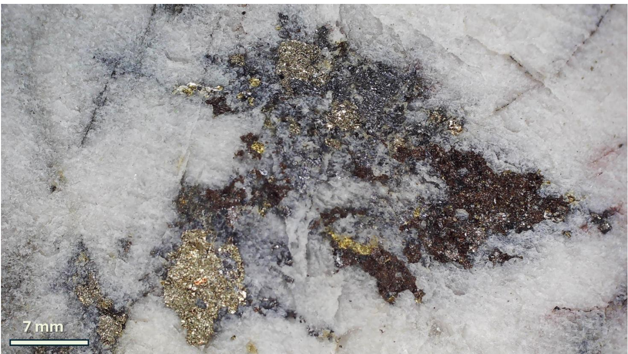
Figure 3: Microscope image of quartz hosted Galena-Sphalerite-Chalcopyrite-Pyrite aggregates hosting Au and Ag mineralisation (0.3m @ 1.91g/t Au and 650g/t Ag from 192m) hole 25NED004.
