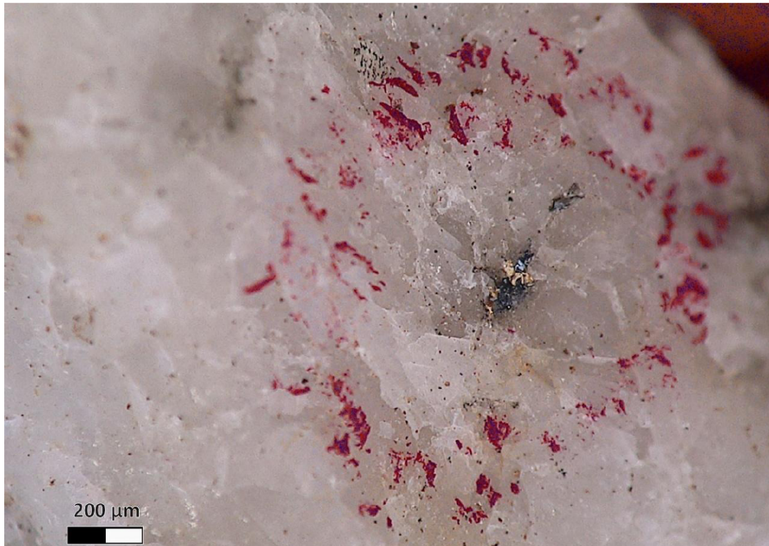
Figure 2: Visible gold in rock chip sample 387032 at Invincible which returned 7.32 g/t Au (refer Table 1).
