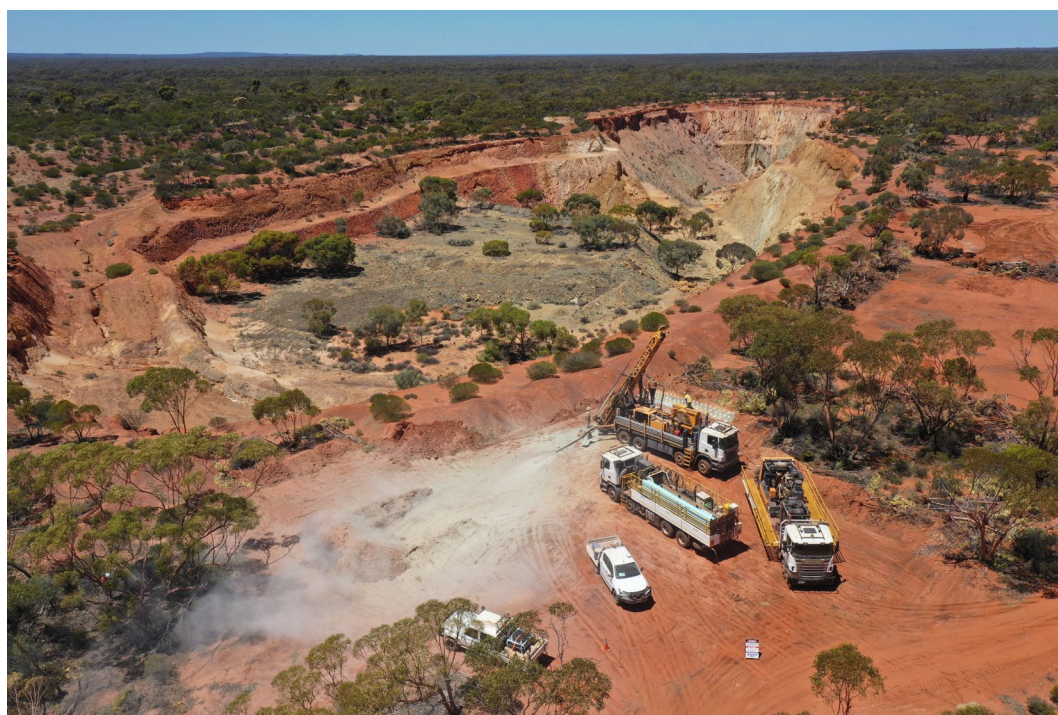
Figure 1: JBell RC Rig drilling with the Lizard historic Pit in the background
