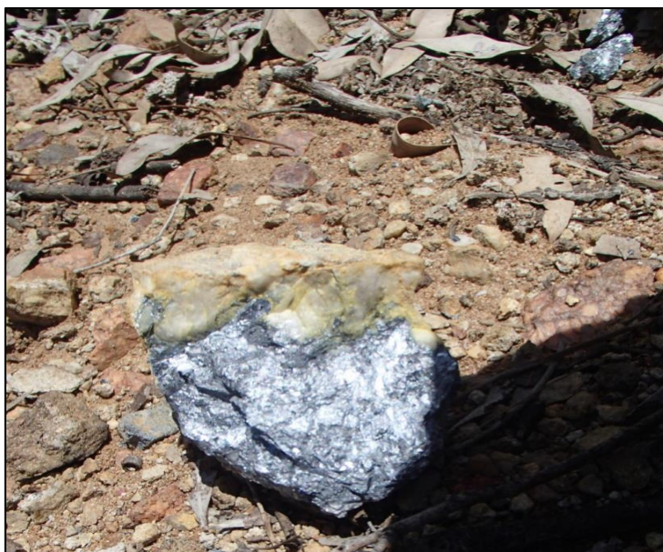
Figure 8: Banshee mine waste dump material observed (unsampled) by Dart Mining in January 2025 showing antimony mineral (70% stibnite*) with encasing vein quartz.*
